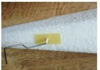
Insert the control horn in the elevator onto the pushrod Z-Bend and place the horizontal stabilizer on the fuselage according the center line.
