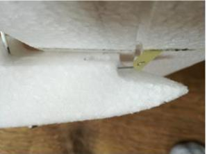
Glue the vertical stabilizer after the glue on the horizontal stabilizer is dry. First glue it to the fuselage and check that it follows the center line of the fuselage and is perpendicular to the horizontal stabilizer. Then glue the tail landing gear wire to the underside of the rudder with the installed plastic tube. Slide the longer control horn onto the pushrod Z-Bend and glue it also to the bottom side of the rudder.
