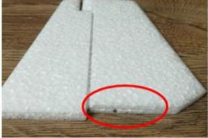
Prepare one more channel in the right-side fuselage part for the servo cables that go from the wing to the receiver, see picture.
