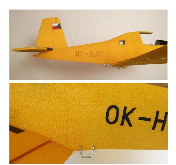
It is recommended to attach wire to the wing ends from below to protect them from contact with the ground.
