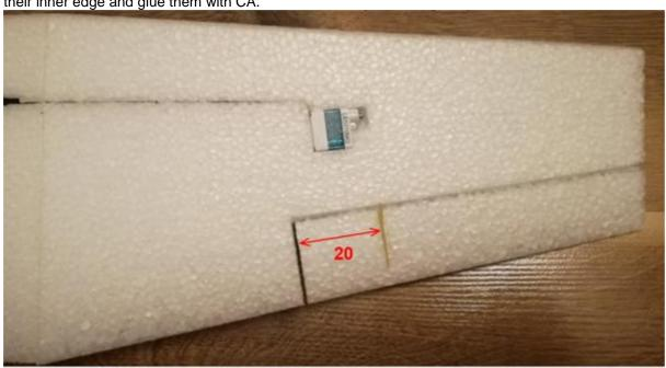
Choose the position of the servos so that their levers are flush with the control horns and have a distance of about 20-25 mm from the "hinge".
