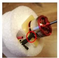
Connect the motor ideally with connectors to the ESC and check the correct direction of rotation. Hollow out a small opening for the cables in the engine cowling and attach it with a few drops CA to the fuselage. Paint the engine "shutters" silver and press them after painting the model in the cowling. The shaft of the motor should come out approximately in the center of the "shutters" with the correct side-thrust and down-thrust.
